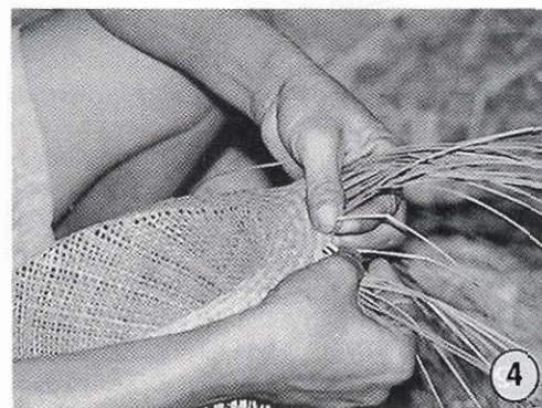
Fig. 2. Processing and weaving of jipi in Becal, Campeche, Mexico. Stripping jipi leaf segments for weaving.
